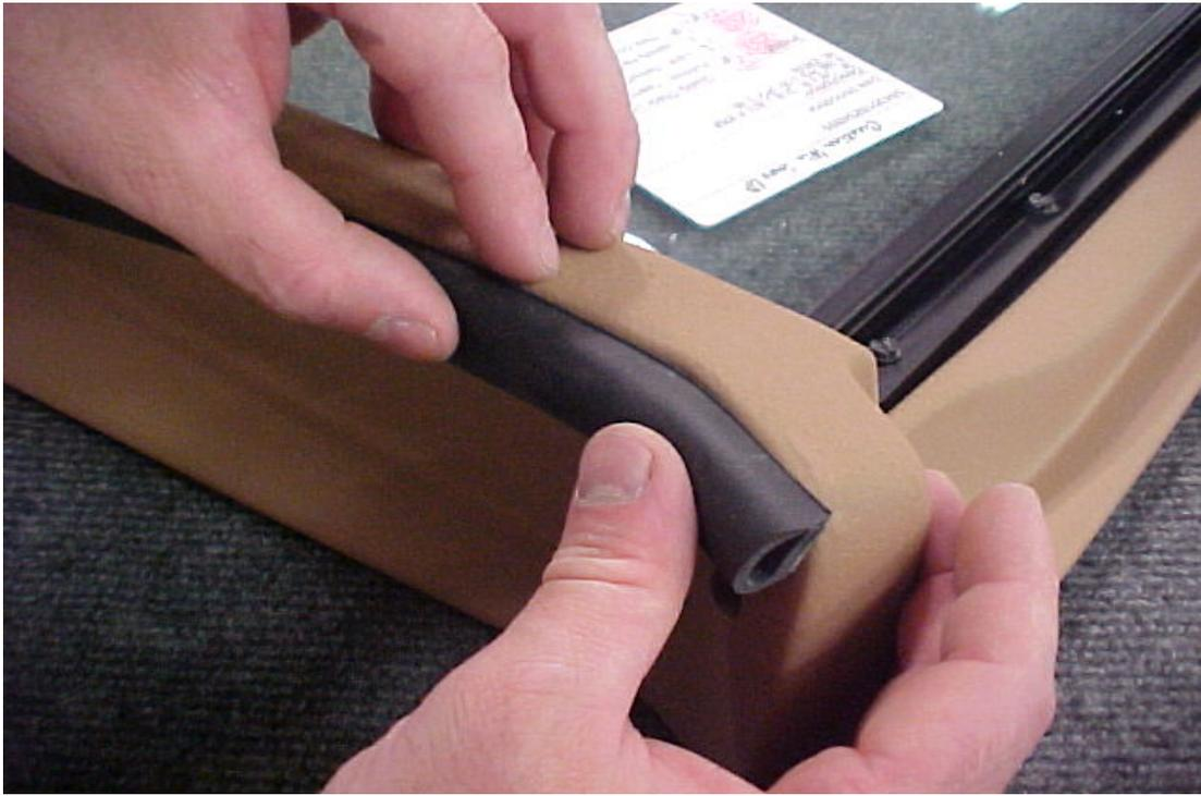
4) Trim off any excess gasket with a razor blade.
