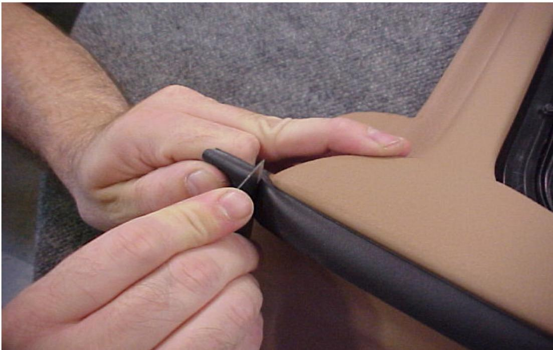
**Perimeter Door Sealing Gasket** – This is the long gasket (approximately 70” in length) that goes around the perimeter of the inside of the door.
